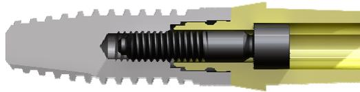
Figure 2 – implant/abutment set with internal hexagon connection “section view”
