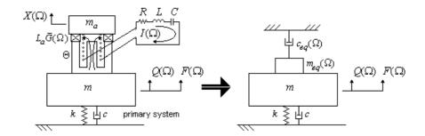
Figure 2. Equivalent quantities for the electro-viscoelastic vibration neutralizer
