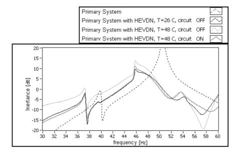
Figure 8. Composite system frequency responses
