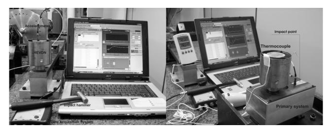
Figure 6. Neutralizer inertance measurement scheme (left) and composite system inertance measurement scheme (right)
