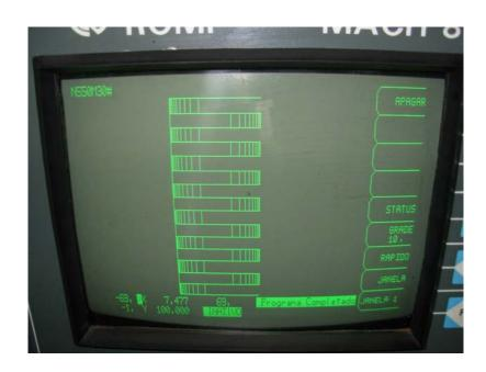
Figure 8 - Graphic simulation of the circular cavity (X, Y)
