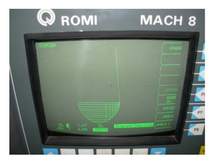
Figure 9 - Graphic simulation of the circular cavity (X, Z)
