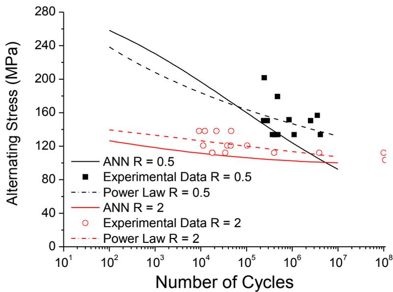
Figure 6. S-N curve of the MAT (0)<sub>2</sub> for R = 0.5 and R = 2, comparing the experimental data obtained from the literature, the data obtained by the ANN and the data obtained by the power law, trained with 3R.
