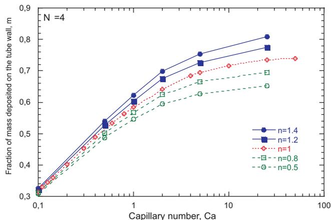
Figure 4. Fraction of mass attached to the wall as a function of the Capillary number with a fixed viscosity ratio,  $N_\eta = 4$ , for different values of the power-law index,  $n = 0.5, 0.8, 1, 1.2,$  and  $1.4$ .
