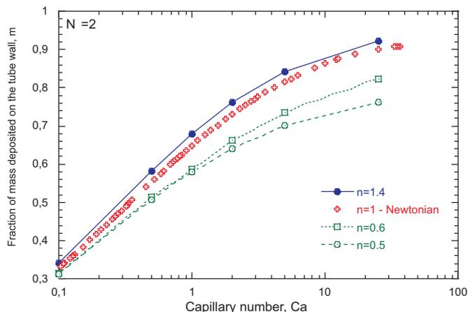
Figure 5. Fraction of mass attached to the wall as a function of the Capillary number with a fixed viscosity ratio,  $N_\eta = 2$ , for different values of the power-law index,  $n = 0.5, 0.8, 1, 1.2,$  and  $1.4$ .
