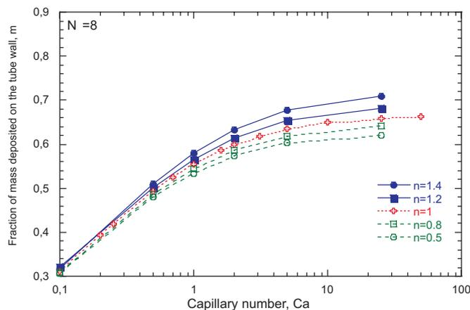
Figure 3. Fraction of mass attached to the wall as a function of the Capillary number with a fixed viscosity ratio,  $N_\eta = 8$ , for different values of the power-law index,  $n = 0.5, 0.8, 1, 1.2$ , and  $1.4$ .
