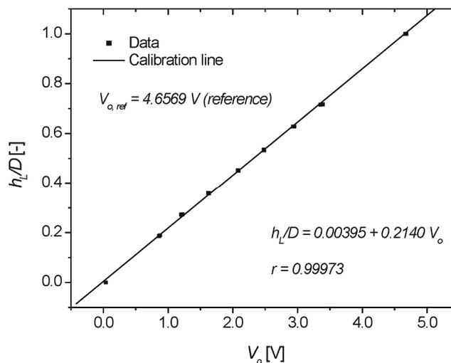
Figure 6. Calibration curves of probe with wires of  $\phi 98 \mu\text{m}$
