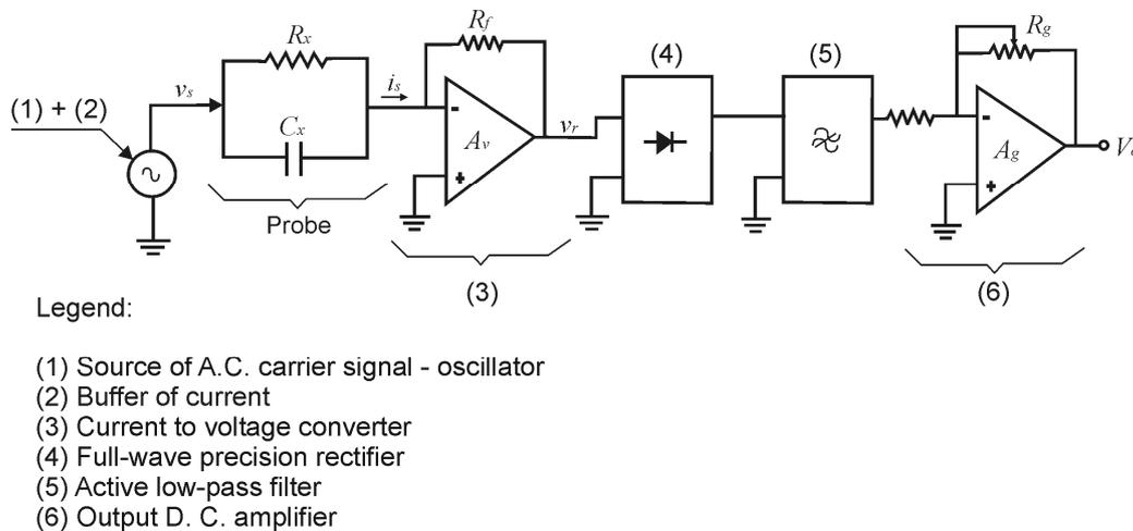
Figure 2. Blocks diagram of the transducer circuit
