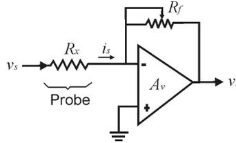
Figure 3. Resistive probe and current to voltage converter
