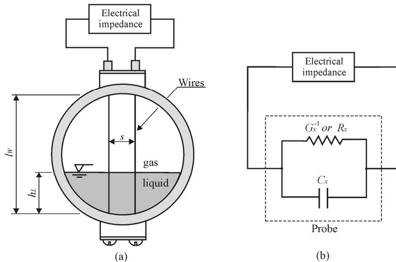
Figure 1. Parallel-wire probe: (a) probe for piping flows; (b) equivalent electrical circuit
