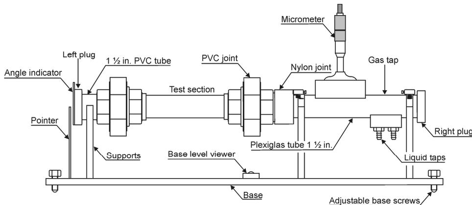
Figure 5. Static calibration device
