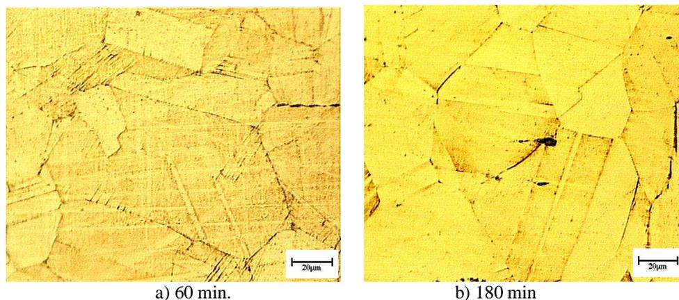
Figure 6. Optical micrograph (500X) of treated sample at temperature 1000°C with treatment time: a) 60 min. and b) 180 min. source: <sup>(4)</sup> adapted.
