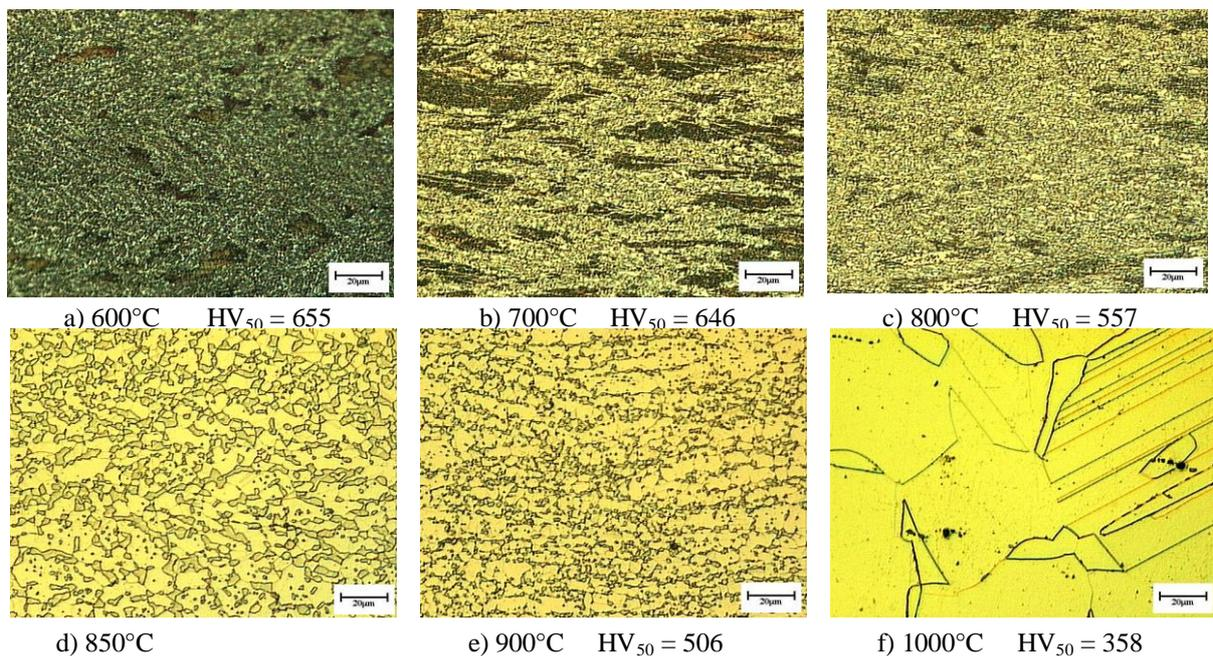
Figure 2. microstructure variation of a Fe-Mn-Al alloy observed of shoulders region under tensile with  $V_c = 0.5\text{mm/min}$  tested specimen at each temperature.
