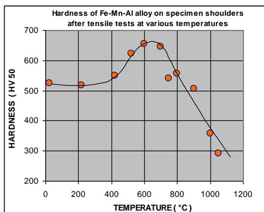
Figure 1. Hardness variation of a Fe-Mn-Al alloy observed on specimen shoulders, after tensile testing at various temperatures, i.e. under test at each temperature.
