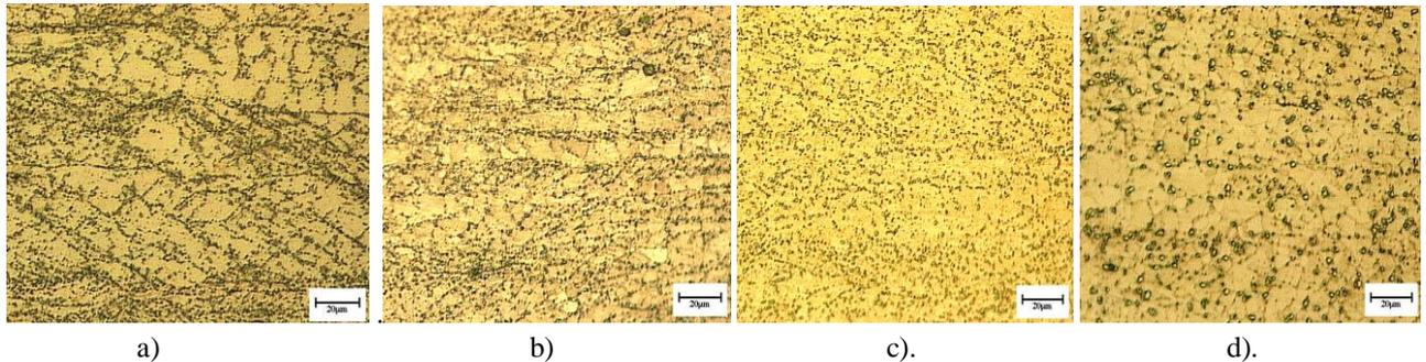
Figure 5. austenitic Fe-Mn-Al (SR) steel heat treated sample at 900°C, with time: a) 5 min.; b) 20 min.; c) 60 min. and d) 180 minute, source: <sup>(4)</sup> adapted.
