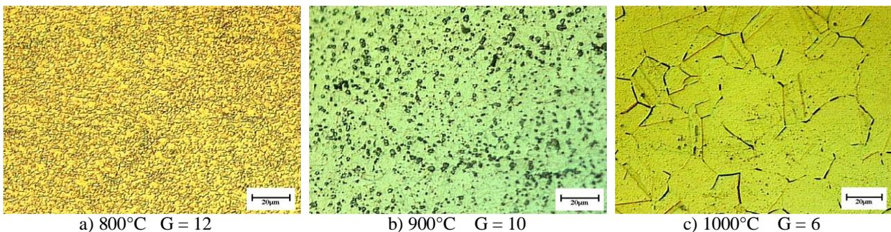
Figure 6. tensile with change  $V_C$  test microstructure of SRA2 material at temperature and grain size (ASTM) of respectively: a) 800°C, G = 12; b) 900°C, G = 10; c) 1000°C, G = 6.
