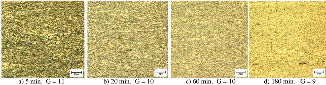
Figure 4. Sample micrograph of austenitic Fe-Mn-Al (SR) steel after heat treatment at temperature 800°C, with time: a) 5 min.; b) 20 min.; c) 60 min. e d) 180 minute, source: <sup>(4)</sup> adapted.
