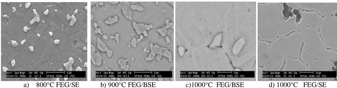
Figure 5. SEM micrography of tensile with change  $V_C$  sample tested SRA2 material microstructure, at temperatures: a) FEG/SE at 800°C; b) FEG/BSE at 900°C; c) FEG/BSE at 1000°C and d) FEG/SE at 1000°C.
