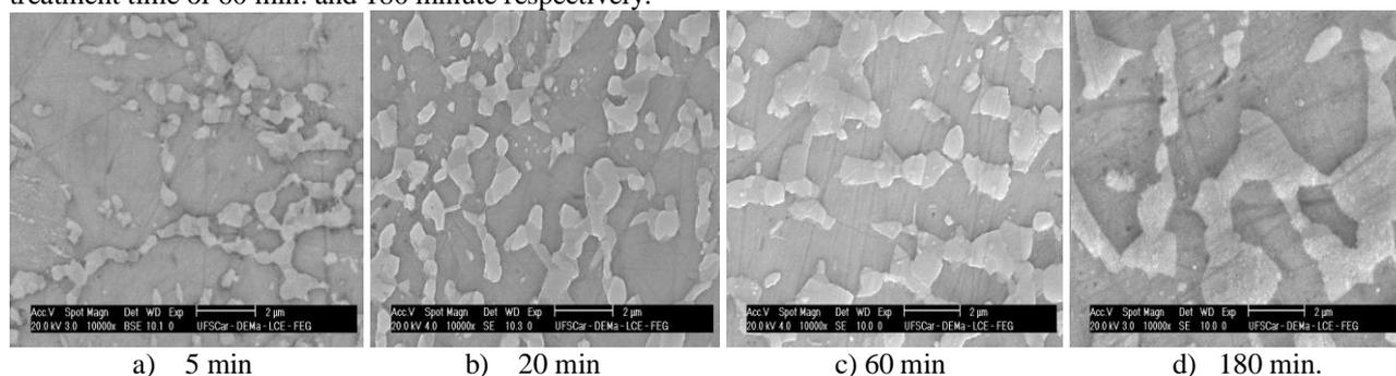
Figure 3 treated sample microstructure of FEG/BSE micrograph at temperature 900°C during: a) 5 min.; and FEG/SE micrograph in: b) 20 min., c) 60 min. and d) 180 min
