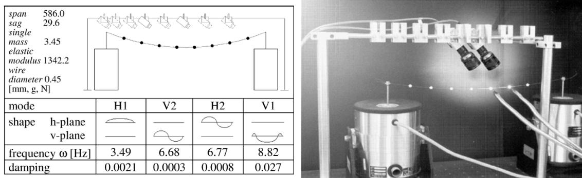
Figure 2. Mechanical model with slacker system parameters and dynamic characteristics; experimental setup.
