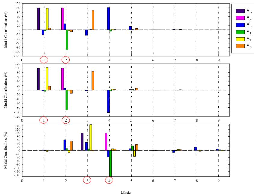
Figure 1. Mode contributions to various nonlinear interaction coefficients:  $\theta=30$  (upper, lower), 45 (middle) deg;  $\lambda/\pi=2$  (upper, middle), 4 (lower).
