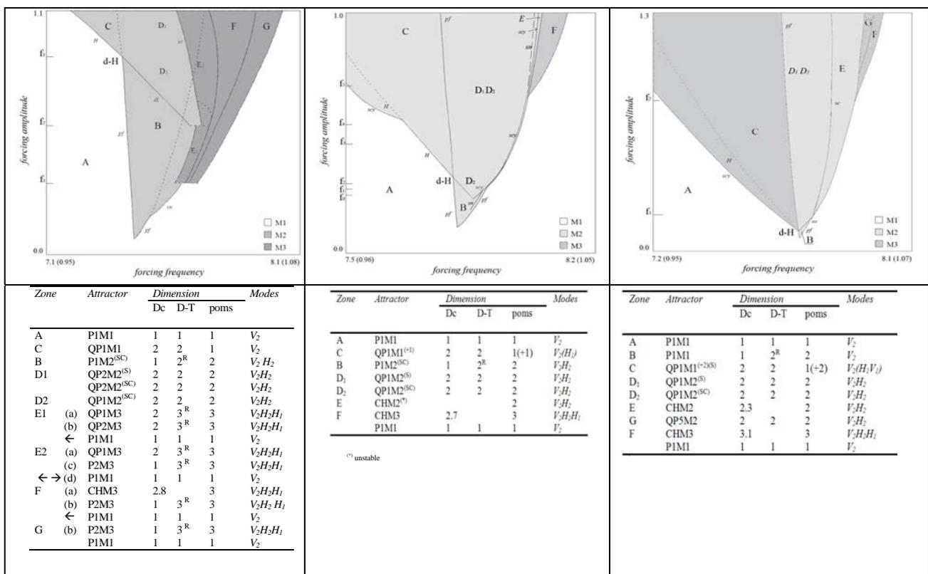
Figure 3. Response charts at various temperatures ( $T=12^\circ\text{C}$ ,  $6^\circ\text{C}$  and  $4^\circ\text{C}$  in first, second and third column, respectively) with zones of periodic (P), quasiperiodic (QP) and chaotic (CH) response, and with qualitative and quantitative characterization of the relevant classes.
