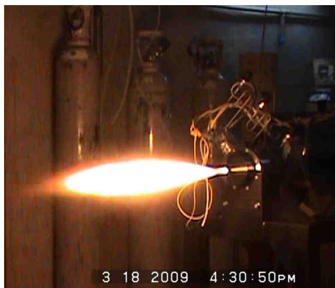
Figure 11. Exhaustion plume of the hybrid thruster.
