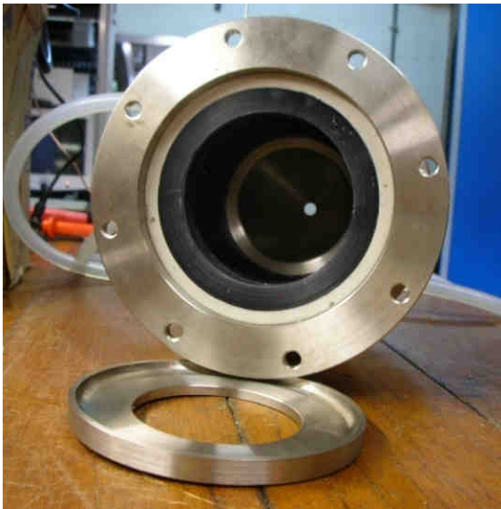
Figure 3a. Hybrid thruster chamber with grain.
