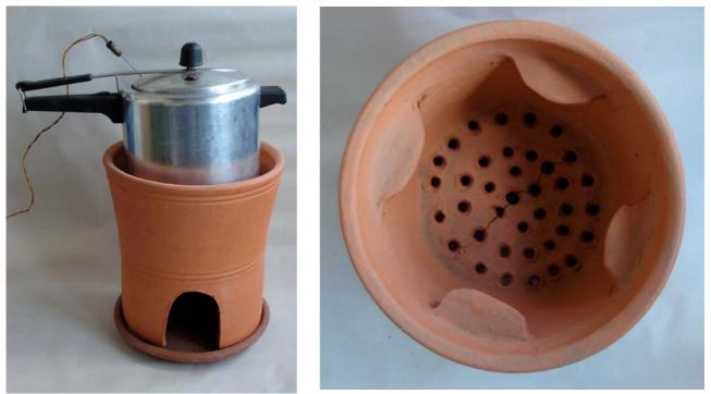
Figure 2. Prototype of the Charcoal Stove (front view and top view)
