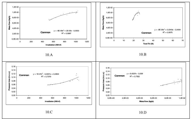
Figure 10. Dynamic behavior of solar collector of 30° tilt and 0.70 m of unevenness.
