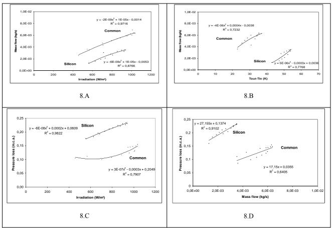
Figure 8. Dynamic behavior of solar collector of 30° tilt and 0.20 m of unevenness.
