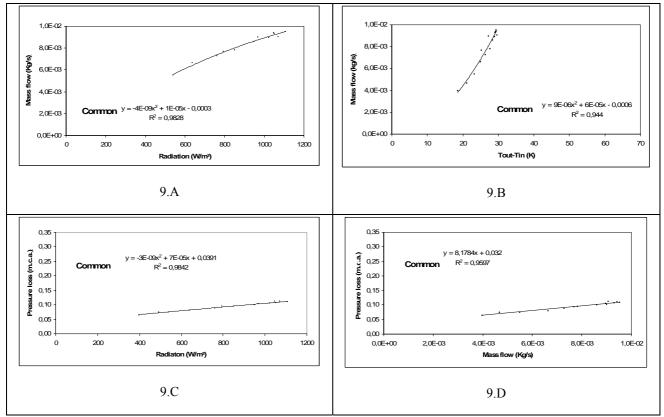
Figure 9. Dynamic behavior of solar collector of 30° tilt and 0.40 m of unevenness.
