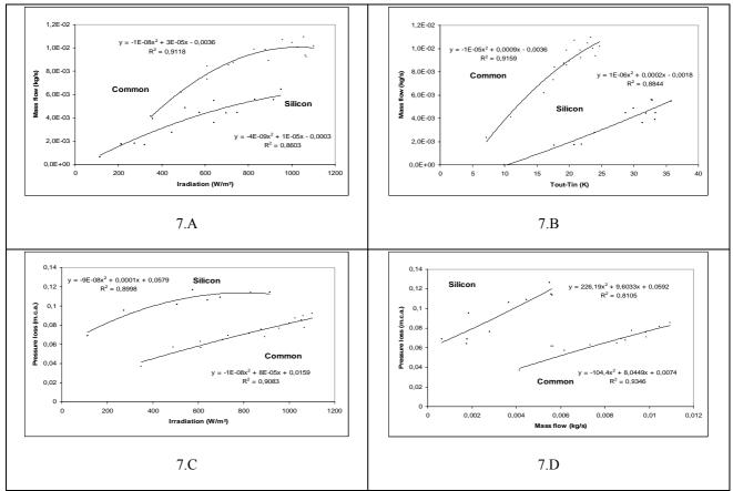
Figure 7. Dynamic behavior of solar collector of 25° tilt and 0.70 m of unevenness.
