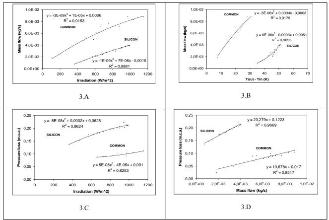
Figure 3. Dynamic behavior of solar collector of 20° tilt and 0.40 m of unevenness.
