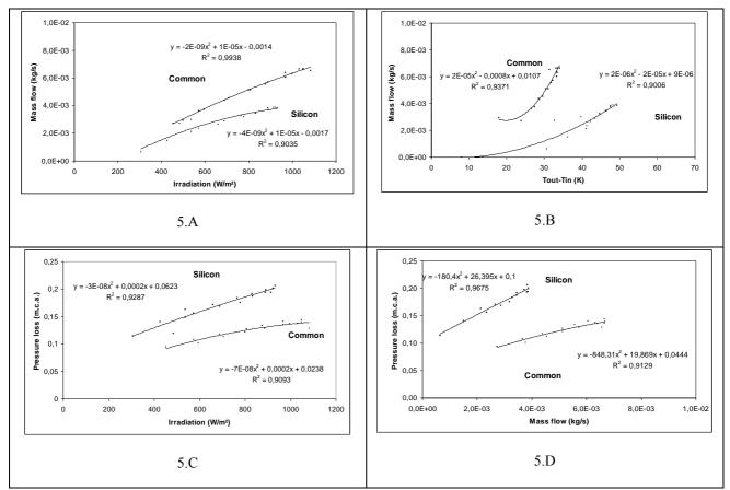
Figure 5. Dynamic behavior of solar collector of 25° tilt and 0.20 m of unevenness.
