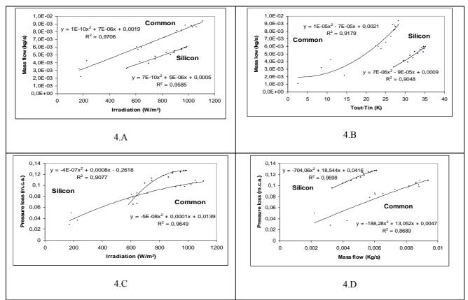
Figure 4. Dynamic behavior of solar collector of 20° tilt and 0.70 m of unevenness.
