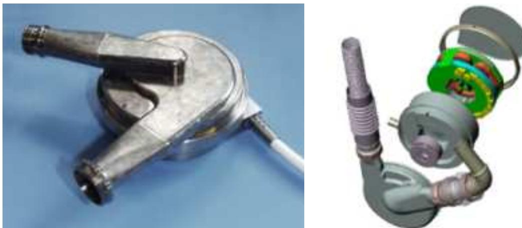
Figure 3-2. Picture and assembly of HeartMate III™
