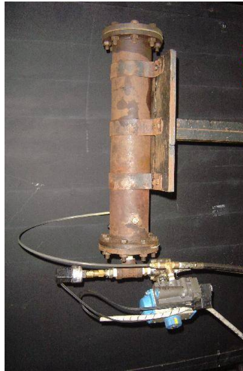
Figure 4. Rocket and main subsystems prior to firing in the vertical stand.
