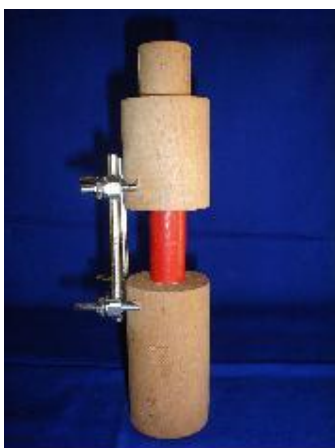
Figure 2: Group 2 model, an internal fixator combined with a wood graft
