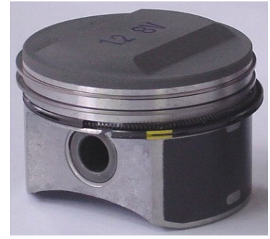
Fig. 5. 15:1 compression ratio piston
