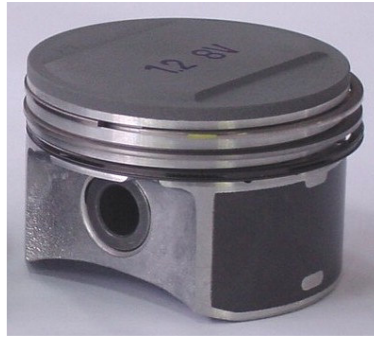
Fig. 4. 12.5:1 compression ratio piston
