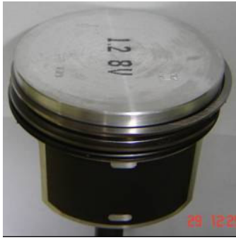
Fig. 3. 11:1 compression ratio piston
