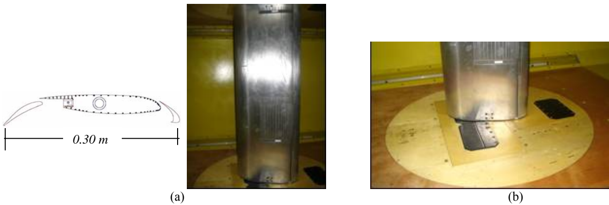
Figure 1. (a) airfoil EMBRAER170 with slat and flap, (b) blowing injectors location at lower wall.
