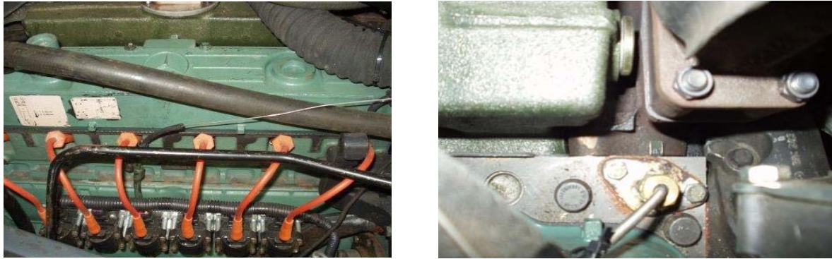
Figure 8. Inserted thermocouple in the block of the engine through rod of oil support (left) and inserted platinum electrical resistance in the liquid of cooling engine block exit (right).
