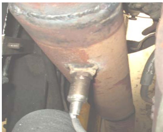
Figure 7. Broad band Lambda sensor installed in exhaust system.
