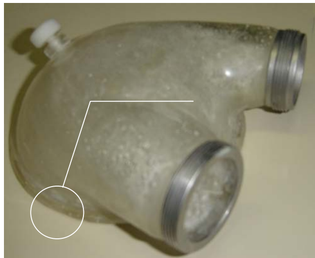
Figure 1. ATAH's chamber with the area that was encountered formation of cracks in evidence.
