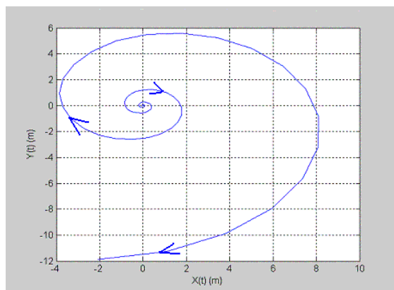
Figure 14. Journal center trajectory for an unstable example at 4,000rpm and 2\omega C_{xx}/K_{xy}=1 .
