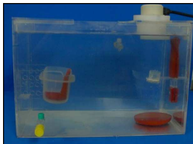
Figure 3. Experimental Bench. At left is the compartment for treatments without ultrasound. At right, ultrasound transducer, polyethylene tube, support and rubber.
