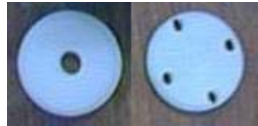
Figure 5. Inserts from which cold air (left) and hot air (right) flows through before leaving the vortex tube
