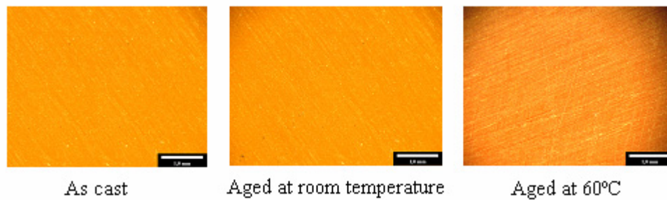
Figure 7. Micrographs of the surface in the samples before and after hygrothermal ageing.
