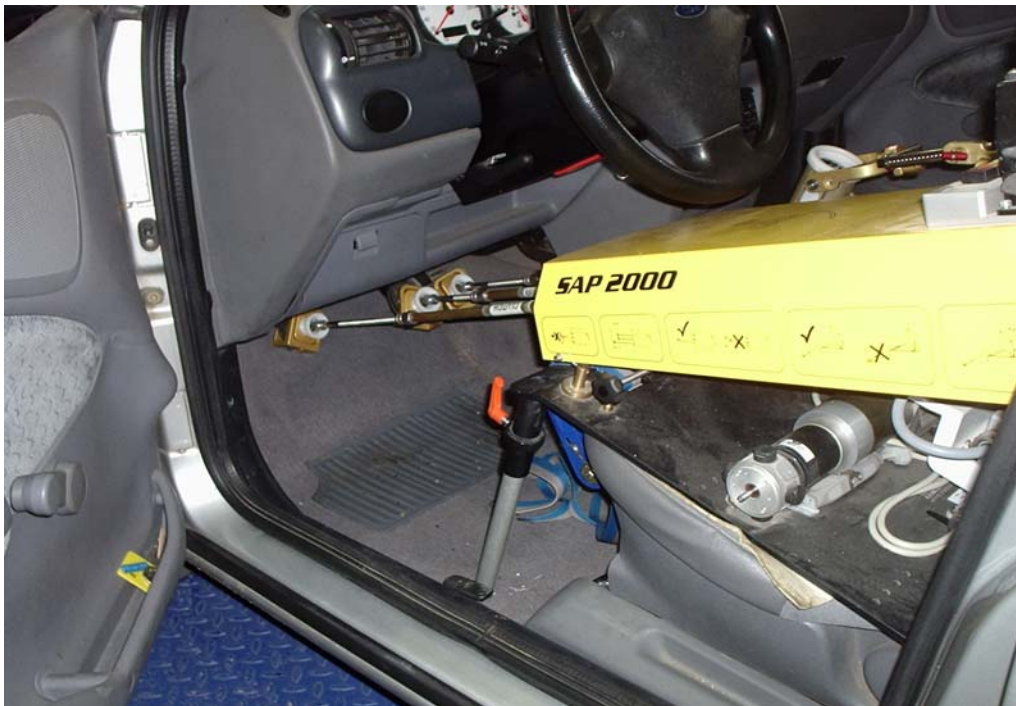
Figure 3. Detail of pilot-robot "legs" operating the accelerator, brake and clutch
