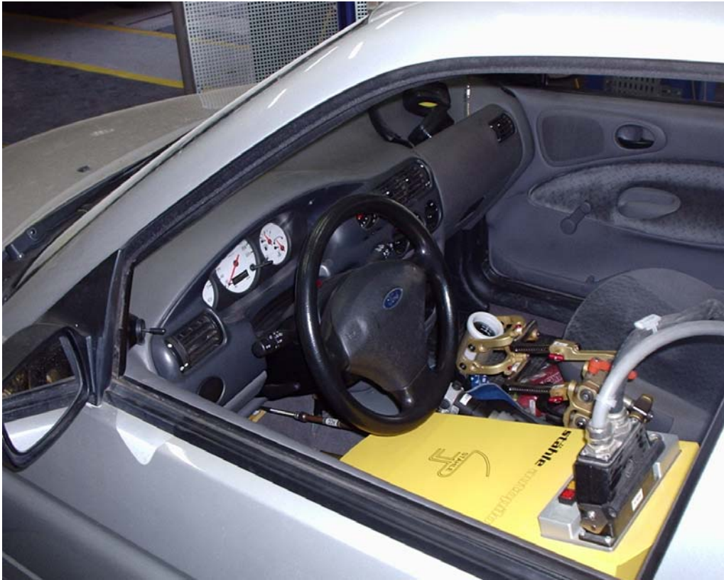
Figure 2. Pilot-robot installed in the vehicle showing the detail of its mechanism for gear box change
