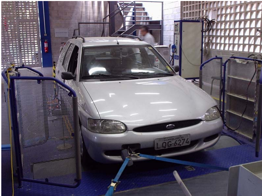
Figure 4. The vehicle utilized for tests positioned on the chassis dynamometer
