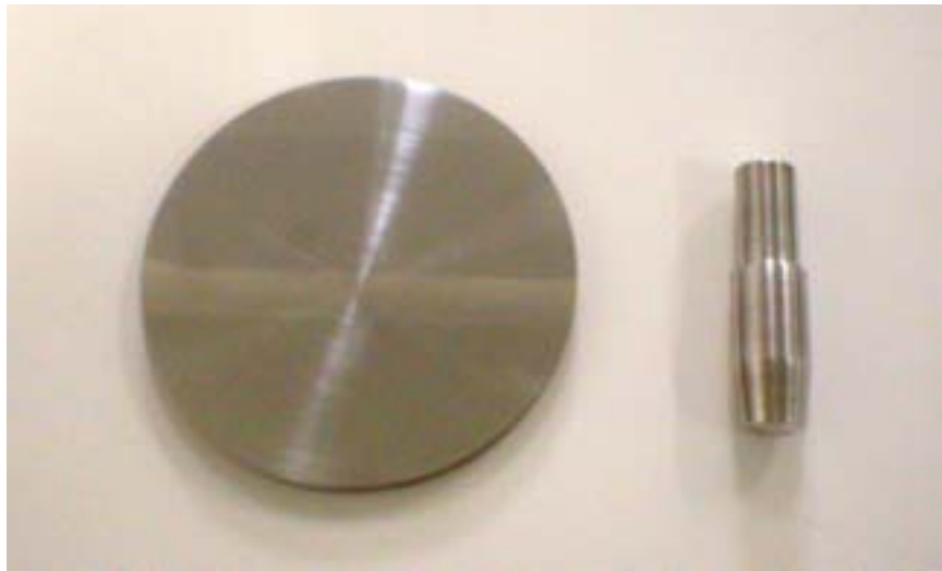
Figure 2. Gray cast iron disc or counterface and steel pin for testing in the pin-on-disc apparatus.
