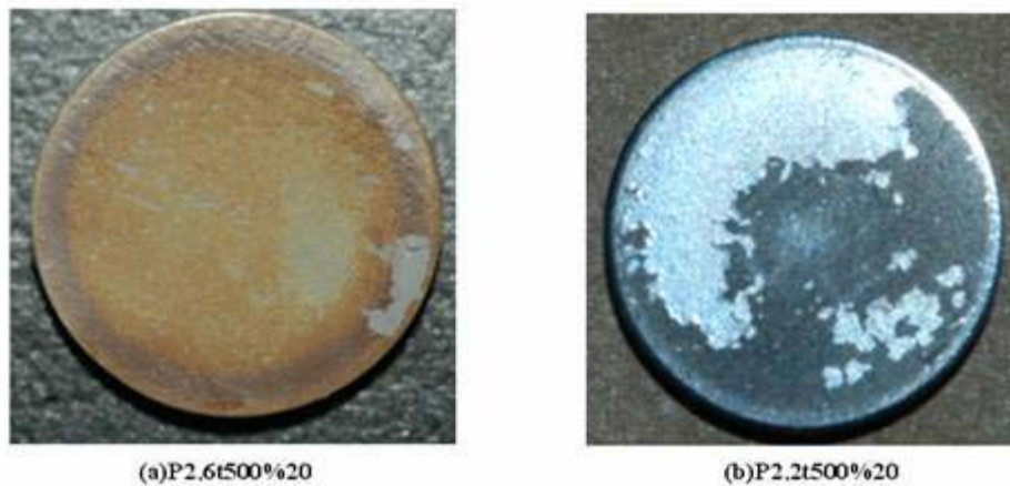
Figure 3. Oxide layer partially detached from Ti surfaces.
