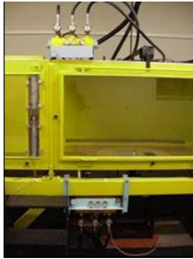
Figure 2. Test section with the compressed air supply and control system, rake and a blower.
