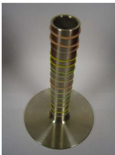
Figure 2 - Cylindrical device for the elastic pre-stretching.
