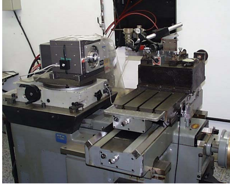
Figure 1. Lateral view of the ultraprecision lathe
