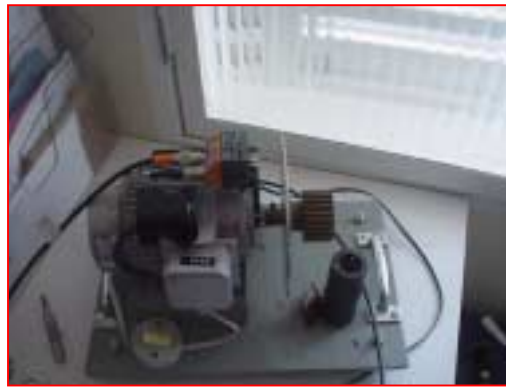
Figure 1 - Electric Motor with defect in the outer race of the rolling element bearing
