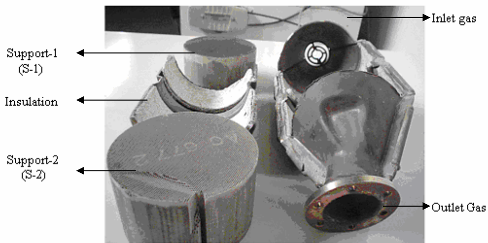
Figure 1. Components of the Catalytic Converter
