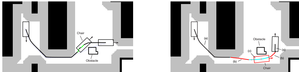
Figure 8. Sample trajectory taken by the wheelchair while in the autonomous mode (left). The solid black line shows when the deliberative controller is invoked. The lighter (green) line segments represent where the activated obstacle avoidance behavior is composed with the deliberative behavior. The dashed (blue) line is the trajectory that the chair takes if there are no obstacles. On the right, a sample wheelchair trajectory using a deliberative plan, combined with user input (semi-autonomous mode). Part(a) represents the deliberative path taken, part(b) represents the user's input, which is consistent with the deliberative plan, part(c) represents when the obstacle avoidance behavior is activated.
