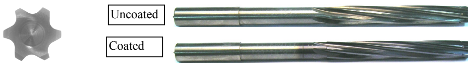
Figure 3. Spiral teeth reamers – tool number 1 and 2 uncoated, 3 and 4 coated
