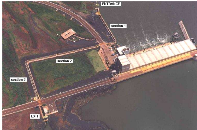
Figure 2. Aerial view of the fish ladder in the IHPP Source: Companhia Energética de Minas Gerais - CEMIG
