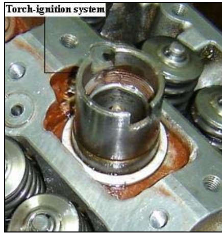
Figure 5 – Torch-ignition system adapted to the engine
