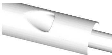
Figure 7. Generic contoured submerged intake (Taskinoglu and Knight, 2002).
