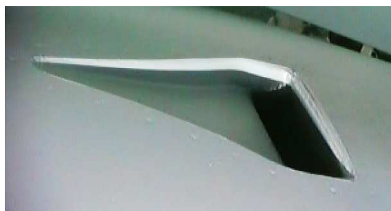
Figure 1. Typical NACA inlet (Faria and Oliveira, 2002).
