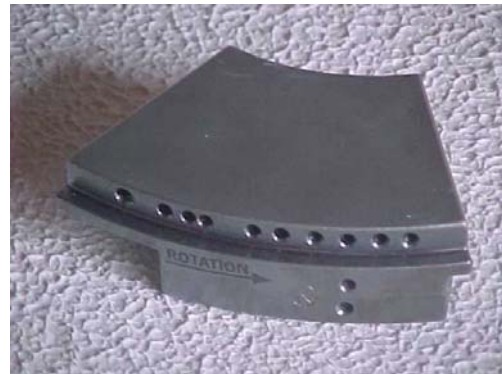
Figure 4. Undersurface and axial thermocouple positions in the pad
