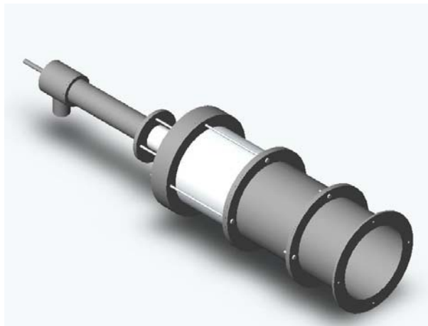
Figure 1. CFD-based virtual image of the LPP Laboratory Model (including a cylindrical UV quartz combustion chamber)
