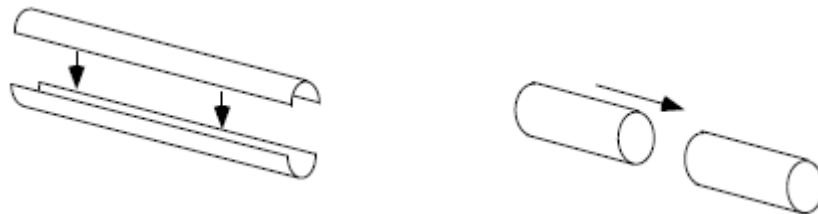
Figure. 1 – Alternatives to Building Aircraft Cylindrical Fuselage Sections
