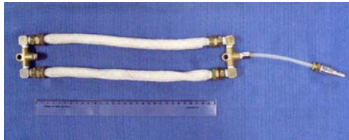
Figure 2 Pneumatic artificial muscle realized at LABBIO.
