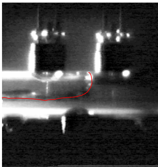
Figure 2 - Gas bubble nose in intermittent horizontal flow of water-air
