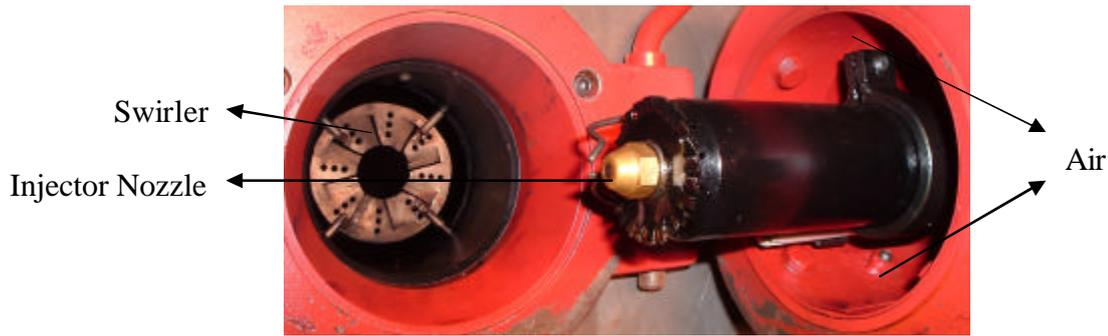
Figure 2. Injector Nozzle.
