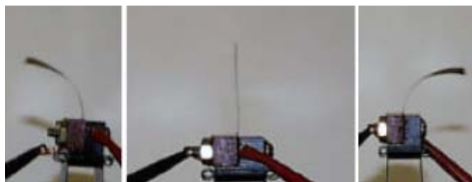
Figure 2. An electrostrictive grafted elastomer-based bimorph actuator in an unexcited state (middle), one direction excited state (left), and opposite direction excited state (right). (Courtesy of Ji Su, NASA).
