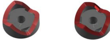
Figure 1. CAD models of the test pieces 1(left), and 2 (right). The top surfaces are those that will be finished with the 3 and 5-axes operations.
