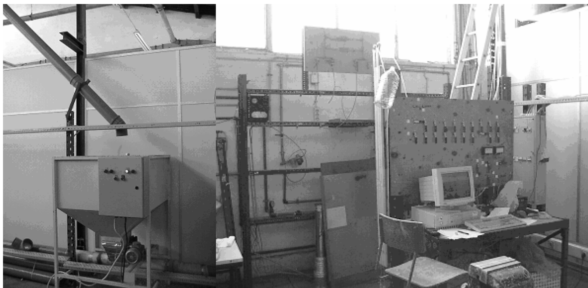
Figure 2. Images of the feeding hopper and of the data acquisition system.
