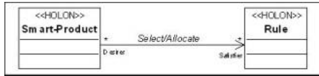
Figure 7. UML diagram of the Holonic Control solution upgraded as a product-driven Holonic Control solution.
